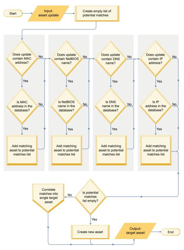
Figure 2. Asset data workflow diagram
